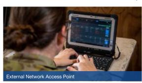
One of the revolutionary features of the system is the External Network Access Point which, for the first time, allows Australian Defence Force personnel to securely communicate using untrusted public networks, such as the internet. It eliminates the traditional restriction of needing to use specific Australian data links, giving deployed forces the ability to securely communicate in anv environment.
