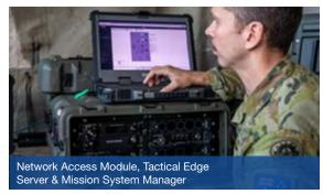
The heart of the system is the Network Access Module (NAM) - a rugged hardware case which provides the power and services needed to enable secure communications. Under the initial LAND 2072 Phase 2B acquisition contract, the NAM provided for up to six capability 'bricks' to be plugged into the case depending on the mission's need. This is being expanded through the Capability Enhancement Program, with additional bricks under development to respond to the evolving threat environment. Unlike
