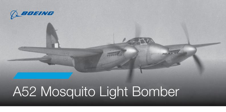
The de Havilland DH 98 Mosquito was one of the greatest combat aircraft of World War II. Originally conceived as a fast, unarmed, light bomber that would be able to outfly fighters, the lightweight, all-wood construction "Mossie" first flew on Nov. 25, 1940, and had a top speed of almost 400 mph. Mosquitoes were built in several different versions, including fighter-bombers (FBs), photo-reconnaissance, day and night bombers, and long-range day and night fighters.
