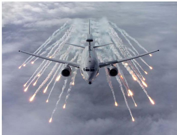
*A 737 AEW&C aircraft releases flares during the Counter Measure Dispenser System tests*
