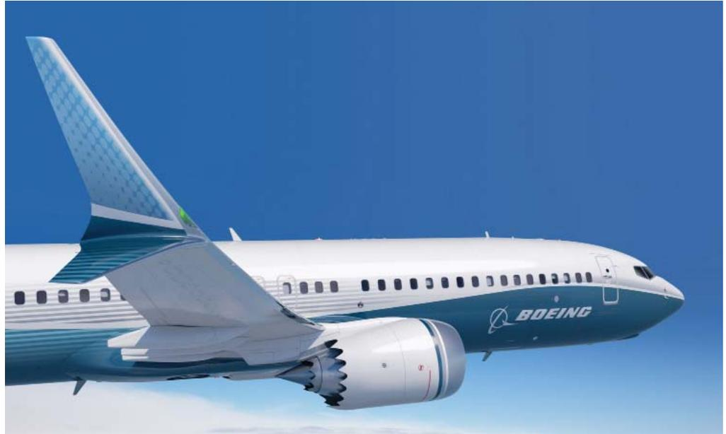
Boeing has unveiled a new winglet design concept for the 737 MAX. The new Advanced Technology winglet will provide MAX customers with up to an additional 1.5 percent fuel-burn improvement, depending on range, on top of the 10-12 percent improvement already offered on the new-engine variant.
