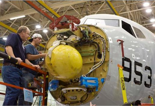
*A Boeing and a Raytheon employee complete installation of an APY-10 radar antenna on P-8A Poseidon test aircraft T2*
