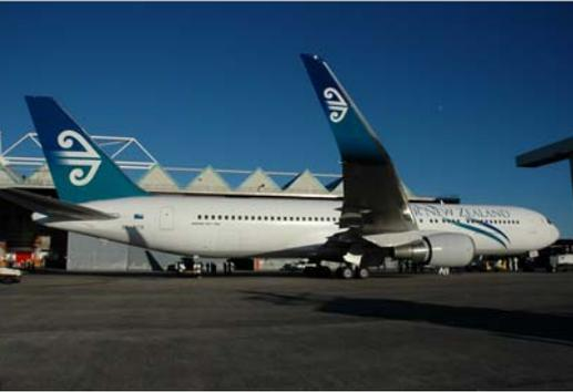
*Above: Air New Zealand has fitted its Boeing 767-300ER aircraft with performance enhancing blended winglets which are estimated to reduce fuel consumption by about six million litres a year and carbon emissions by 16,000 tonnes*
