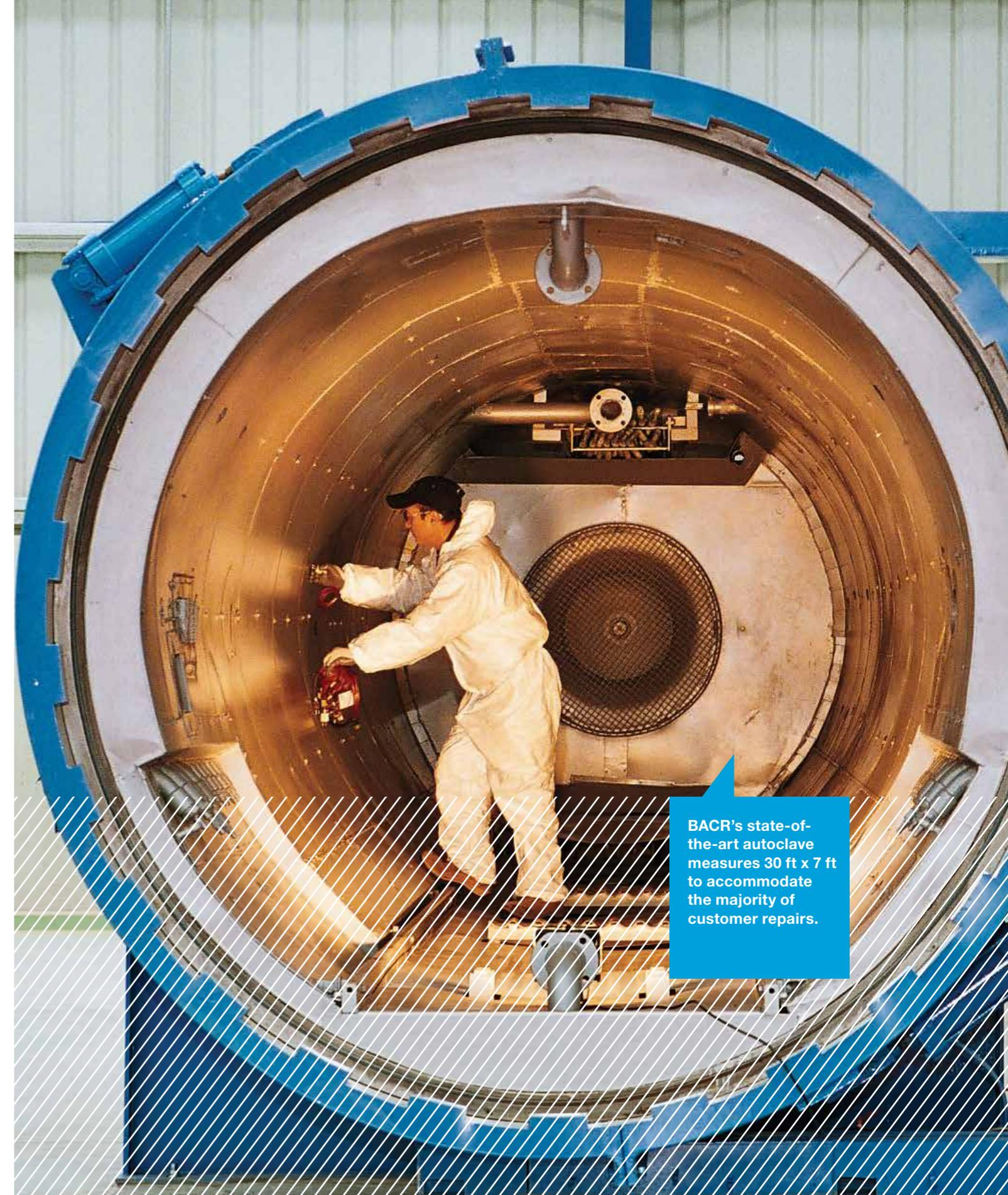
BACR's state-of-the-art autoclave measures 30 ft x 7 ft to accommodate the majority of customer repairs.
