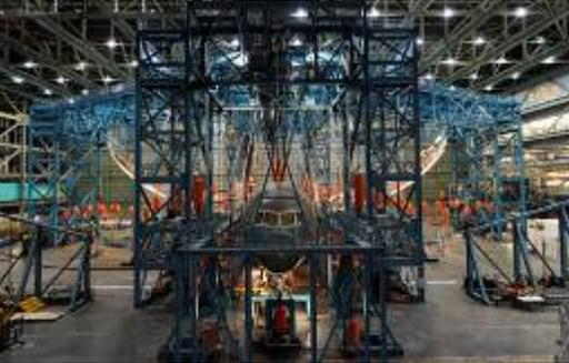
Boeing has successfully met all test requirements during the 787 Dreamliner's ultimate load wing and fuselage bending test. On March 28, loads were applied to the test unit to replicate 150 percent of the most extreme forces the airplane is ever expected to experience while in service. The wings were flexed upward by approximately 7.6 metres during the test and the fuselage was pressurised to 150 percent of its maximum normal operating condition.
